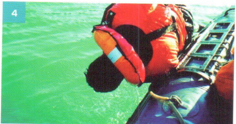
4 The lift takes no longer than 5 seconds due to the cradles 2 to 1 mechanical advantage.
